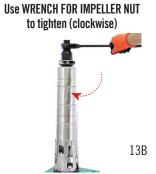
Use TORQUE TESTING NUT and WRENCH to tight at correct torque (clockwise) (Step 7)
