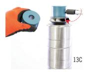
Loosen with Allen Tool, remove from Fixture Seat. Remove 6" Jig with Allen Tool from Assembly
