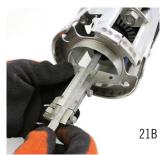
22 Pull out SHAFT using DEPTH TOOL
