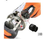
9 Use TORQUE WRENCH and FIXTURE FOR STRAP to tight at correct torque (clockwise)
