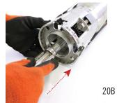
21 Use DEPTH CALIPER to check shaft clearance
