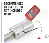
Fit Interconnector and Coupling/Shaft on Jig 6" Motor using 19mm wrench and allen wrench (clockwise)
